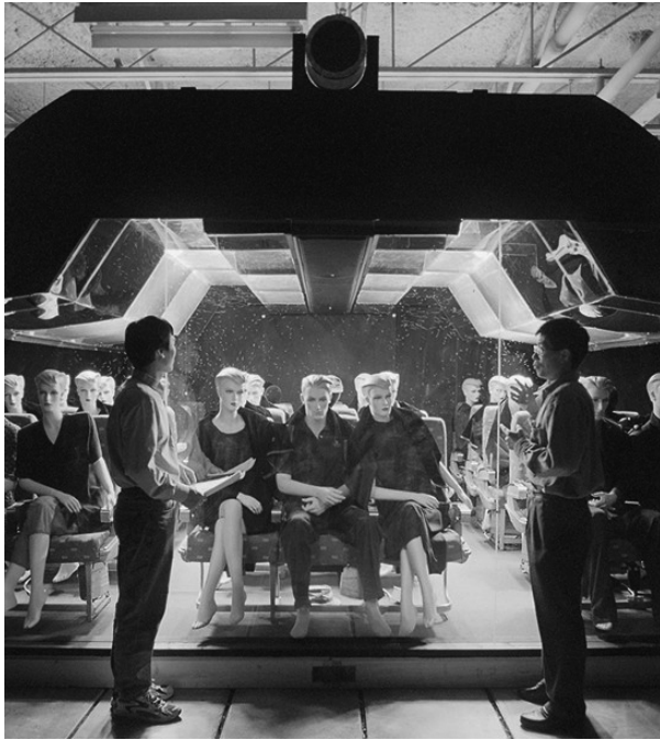
From left, PhD student Yigang Sun and his advisor, Yuanhui Zhang standing in front of a Boeing 767-300 cabin mockup, discussing the volumetric particle tracking velocimetry they developed to measure air flow patterns and pollutant transport.
